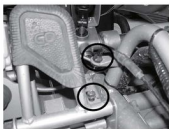
Clearance adjusting nut for throttle Stop bolt for "GO" pedal
